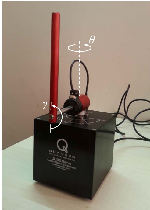
Figure 8: Rotary inverted pendulum apparatus, shown here with \theta \approx 0^\circ and \gamma \approx 180^\circ .
