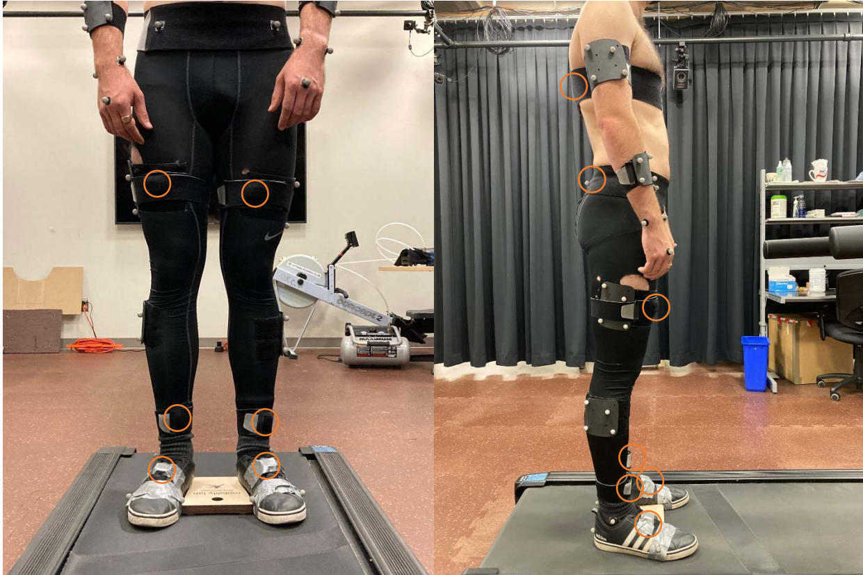
Figure 1. Participant in standing pose on the treadmill showing the dynamic marker set, inertial measurement unit positions (strapped to segments, circled in orange), and the wooden block.
